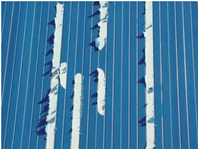
Figure 47. Inter-coat adhesion failure on a prepainted GALVALUME ® panel.
