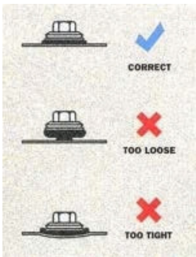
Figure 10. Schematic example of the proper and improper installation of fasteners.
